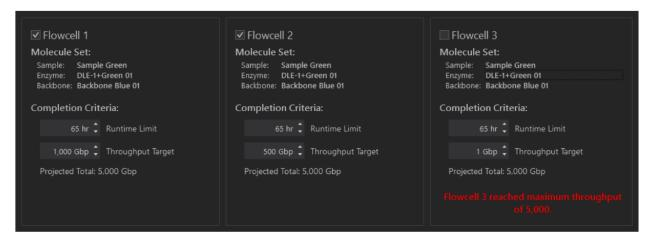
Fig. 4. Error message showing flowcell 3 has reached maximum throughput.
