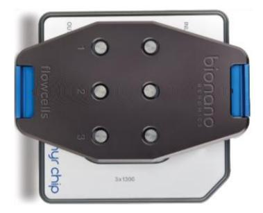
14. The chip and sample can be left out for up to 1 hour at room temperature with the clip engaged before starting the run.
