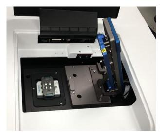
4. Insert one or two chips (if applicable) into the instrument and ensure that it rests snugly on the stage. If only inserting one chip, either platform can be used.
